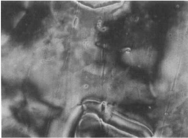
PLATE 8 Twist wall with a wedge disclination of strength -1 , which appeared because of the upward movement of -1/2 nucleus. The other singularity is also found to reach the edge of the wall, 65°C, crossed polaroids, 400×, 12 \mu (See Color Plate VIII at the back of this issue)
