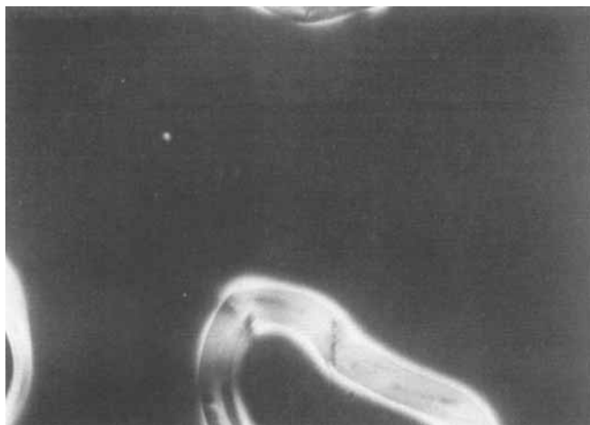
PLATE 5 Twist wall with reversing edge in EBBA, 74°C, crossed polaroids 400 \times , 12 \mu (See Color Plate V at the back of this issue)
